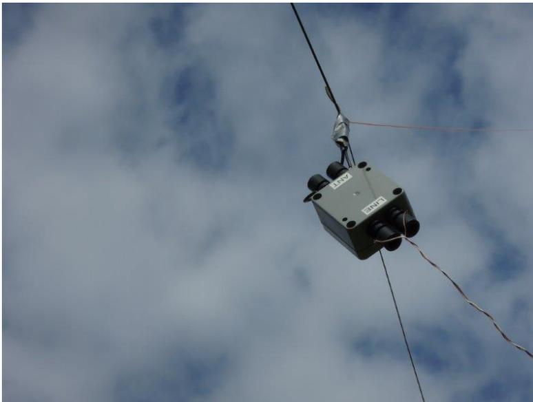
In addition I also built two sets of BOG transformers to experiment with BOG antennas, as this was a new territory for me and I wanted to try it (big thanks to W0BTU for publishing best turn ratios [http://www.w0btu.com/Beverage\\_antennas.html](http://www.w0btu.com/Beverage_antennas.html)). I built one set for using with 50 ohm feedline, the other for 100 ohm feedline (CAT-5).
