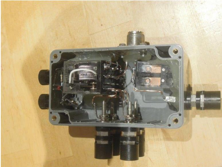
A twisted-pair CAT-5 cable (I have taken a few hundred meters of it) was going to be used to power the relays remotely from home-made TX-RX sequencer. There were going to be some challenges with this arrangement, more on this later.
