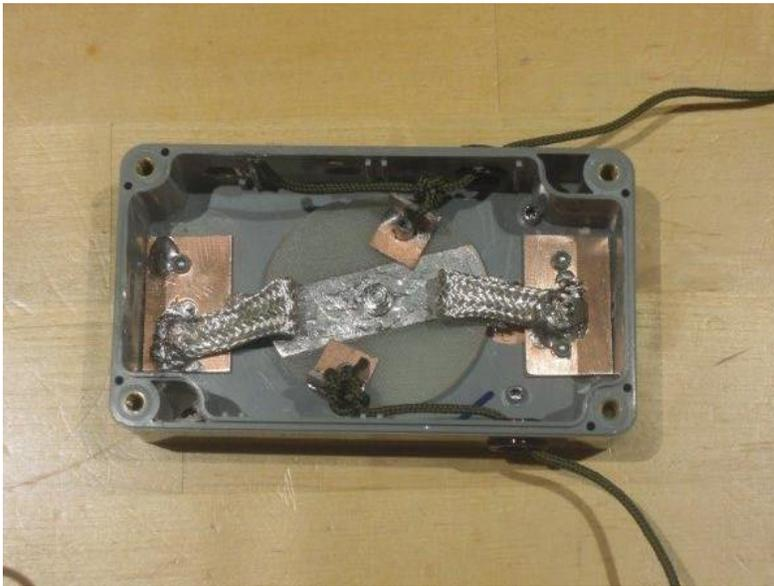
The last night before the departure I have reassessed the convenience (or the lack of it) of walking to the field to change bands and reverted back to an LC trap option, but this time I built it using QRO style Russian transmitting caps. There is plenty of research on the internet suggesting an LC trap will represent lower losses if it is tuned outside the operating freq. I did mine to resonate on 3.7Mhz. This was going to be a major puzzle for me in the field (more on this later).
